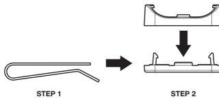
SLIDE BELT CLIP OVER ADAPTER PLATE STEP 2 PUSH SPARE MOUNT ONTO ADAPTER PLATE
